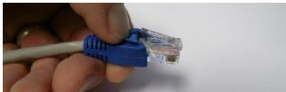
Pull boot back to access lock clip
