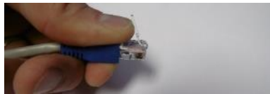
Pull boot back to access lock clip
