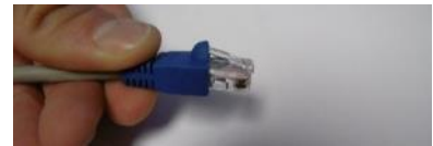
Slide boot back over lock clip
