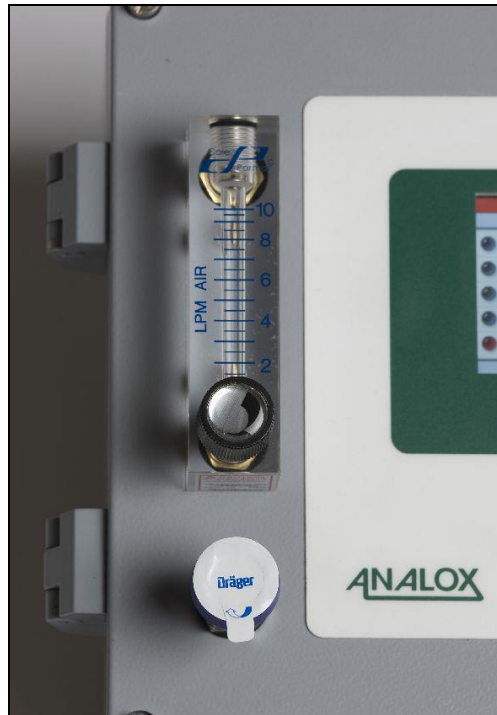
Figure 36 - A Dräger Impactor attached to the outlet port for oil mist testing
