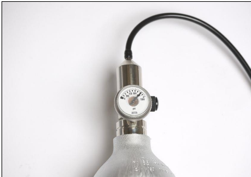
Figure 23 - Flow regulator fitted to calibration bottle
