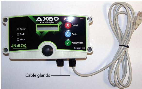
Pre-wired cable for connection to CO 2 Sensor(s)
