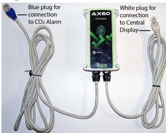
Pre-wired cables for connection to the CO 2 Alarm (left), and to the Central Display (right)
