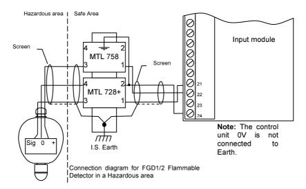
In order to maintain intrinsic safety, the capacitance and inductance or inductance to resistance (L/R) ratio of the loads connected to the terminals of the FGDIO barrier must not exceed specified values:
