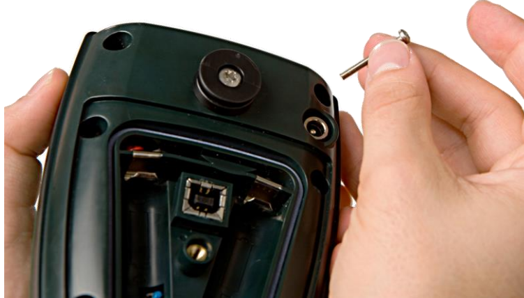
Figure 37 Replace the sensor cap and secure the screws
