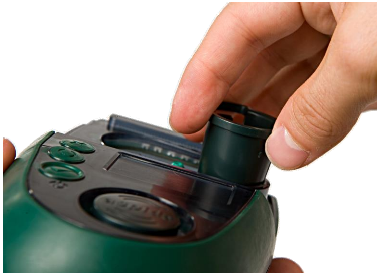
Figure 35 Remove the extraction tool
