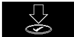
Figure 10 Display shown when the man-down alarm is triggered
