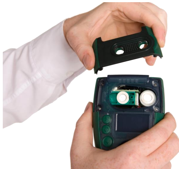
Figure 26 Remove the sensor cap
