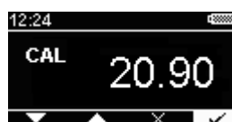
Figure 16 Calibration data entry screen (ready to confirm calibration)
