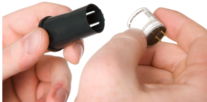
Figure 32 Insert the new sensor into the extraction tool
