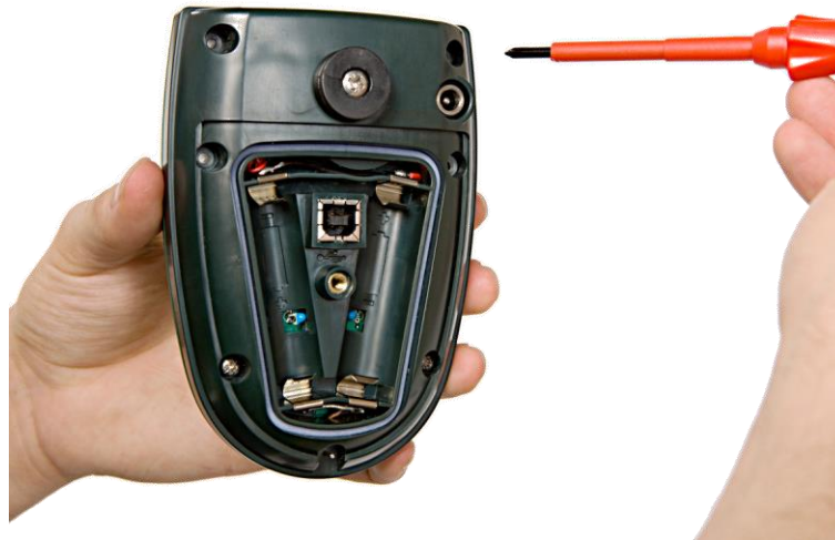
Figure 25 Remove the sensor cap screws
