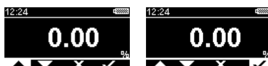
Figure 20 CO 2 LO calibration data entry screen (ready to confirm calibration)
