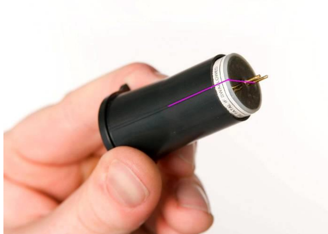
Figure 33 Align the new sensor in the extraction tool
