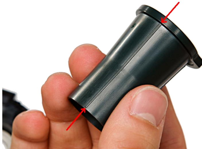
Figure 27 Locate the alignment rib
