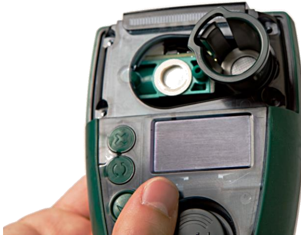
Figure 29 Correct extraction tool position
