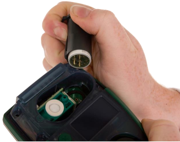
Figure 31 Removing the oxygen sensor
