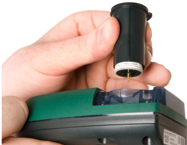
Figure 34 Align the new sensor with the Aspida device
